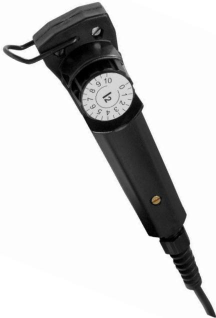
The “Dog bone” style remote control MMA 1 and MMA 3 offer stepless adjustment of the weld current. The adjustment knob can be accessed from both sides making the remote control ideal for both left and right hand operation. The minimum current, as a percentage of the set weld current, can be adjusted in the power source allowing for both Fine and Coarse setting of the current. For more information please refer the power source user manual.
